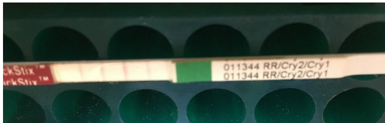
Image of a LFS with three GMO traits identified by marker lines and a control line.
